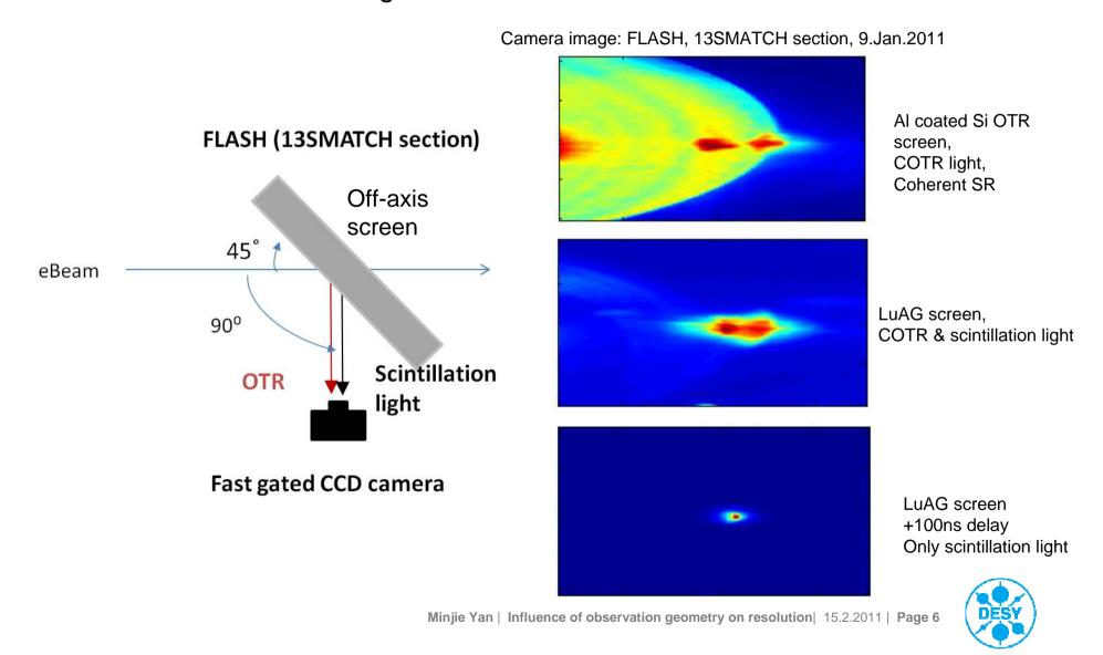
Applicability of scintillation screen in beam profile diagnostics for high-brightness electron beams should be studied.
