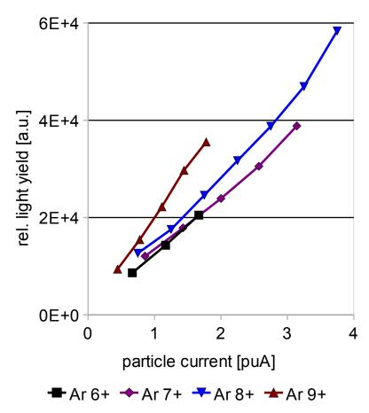
The generated light is linearly growing with the particle current. No saturation effects could be seen in the investigated intensity range.
