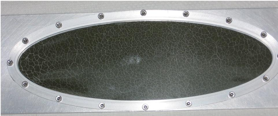
Spectrometer screen in PHIN - the photoinjector test facility for CLIC
