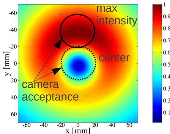
Camera placed to catch maximum light intensity
