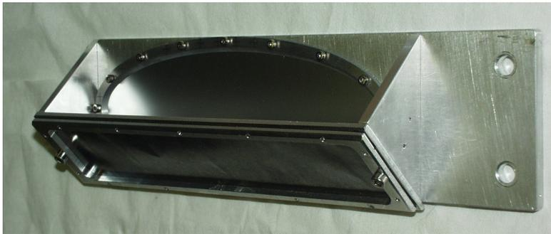
50  $\mu\text{m}$  foil thickness
