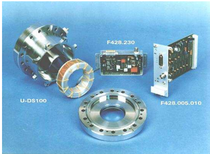
Figure 2.9: Photo of an ac-current transformer used at the pulsed heavy ion LINAC at GSI. The torus with the differential winding is shown left, the used electronic modules at the right.
