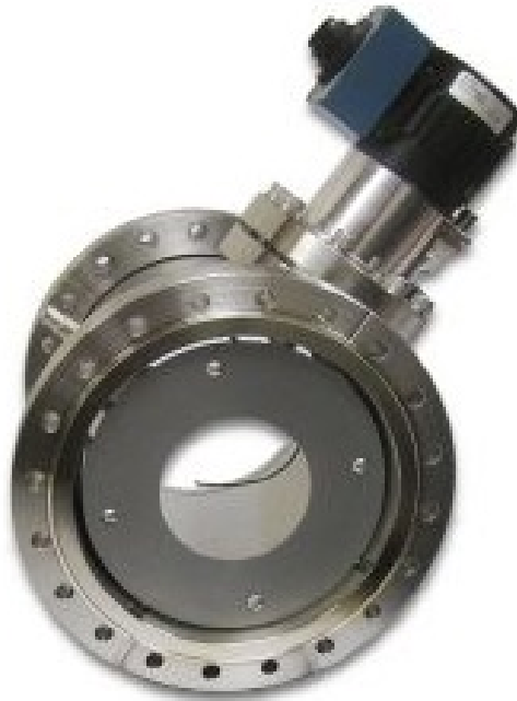
Figure 2.6: Picture of a wire based Beam Position Monitor.
