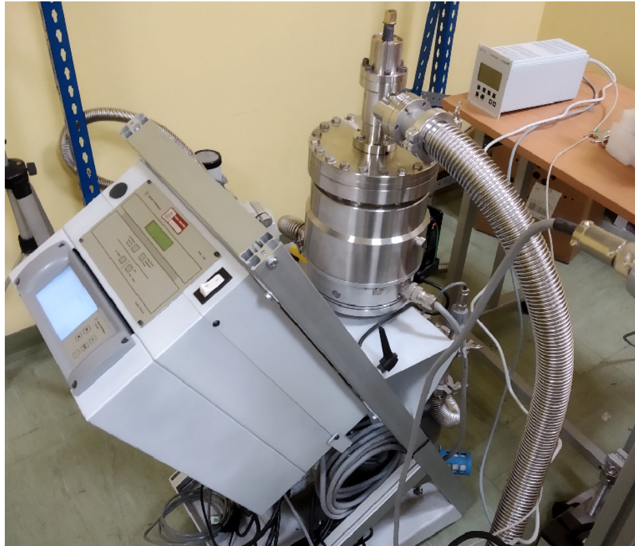
Figure 8.12: Mobile pumping station used in the experiment.
