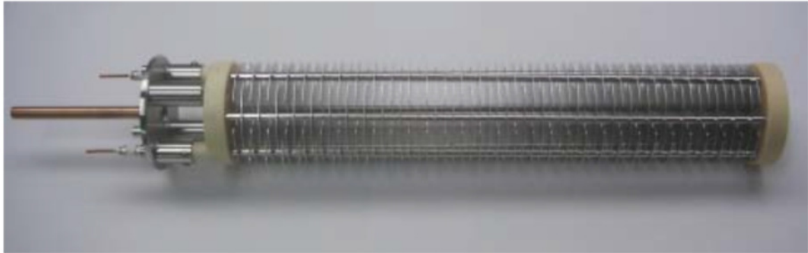
Figure 2.12 – The ionization chamber of an icBLM.
