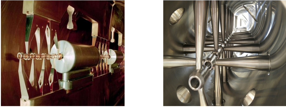
Figure 2.5: The IH cavity TE_{11(0)} - mode (left) [42]. The CH cavity TE_{21(0)} - mode of the FAIR proton linac injector operates at 325 MHz (right) (Courtesy of R. Brodhage).
