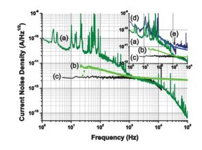
Figure 3: Measured (a) and calculated (b) current noise of the welded pick-up coil with Nanoperm M-764-01 core as well as the measured current noise of the SQUID sensor with rf-shunted input (c). The inset compares the measured (a) and calculated (b) current noise of the welded coil with Nanoperm M-764-01 core with the measured (d) and calculated (e) current noise of the DESY-CCC pick-up coil with Vitrovac 6025 F core.
