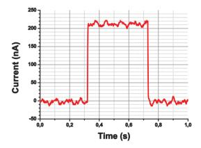
Figure 4: Response of the welded pick-up coil with Nanoperm M-764-01 core connected to the SQUID sensor enclosed into the niobium pots to a rectangular current signal of 220 nA (approximately  $0.5 \Phi_0$ ). There is no low pass filter or time-averaging used. The signal-to-noise ratio is approximately 10.
