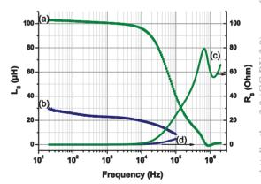
Figure 2: Comparison  $L_S$  (v) and  $R_S$  (v) of the welded pick-up coil with Nanoperm M-764-01 core ((a) and (c)) and the DESY-CCC pick-up coil with Vitrovac 6025F core ((b) and (d)) 4.2 K.
