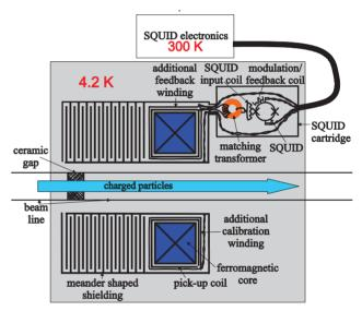
Figure 1: Circuit diagram of the CCC.
