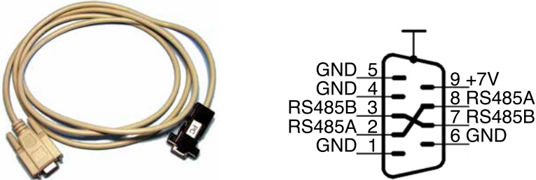
Fig. 18: RS-485 connection. The black plug has to be connected to the COM port of a PC or to an appropriate USB-to-serial converter. Pin assignment shows top view on the connector box.
