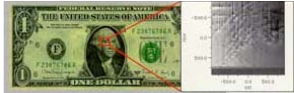
Figure 53 SSM scan of the ink in the region around George Washington's right eye on a one dollar bill.
