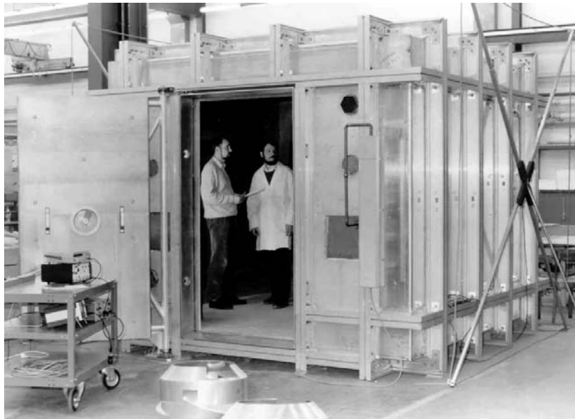
Figure 29 Commercial magnetically shielded room showing first layer of mu-metal shielding and rigid aluminum frame. Courtesy of Vacuumschmelze GmbH.
