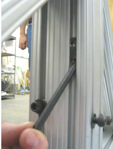
A) Remove one bolt from the washer using the 1/4" hex wrench as support for the washer.
