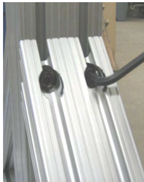
C) Tighten the bolt with the 1/4" hex wrench.
