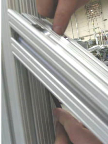
B) Slide the mounting hardware up using the wrench, lining the threads up with the hole and finger tighten the bolt.
