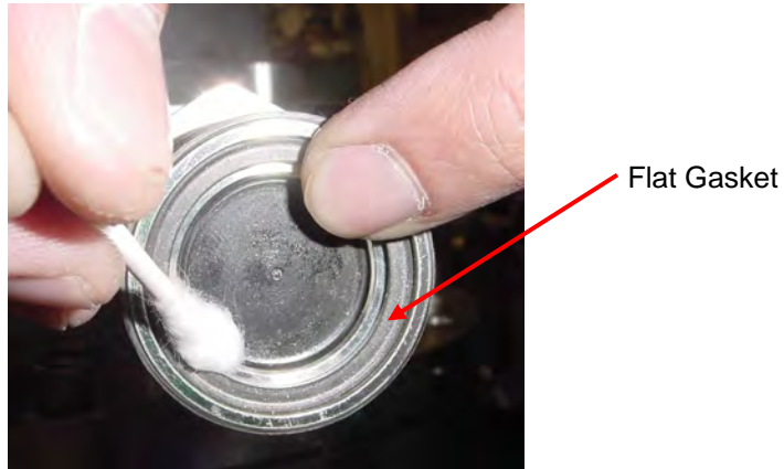
Figure B-2: Cleaning the male Aeroquip®
