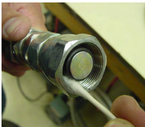
Figure B-1: Cleaning the female Aeroquip
