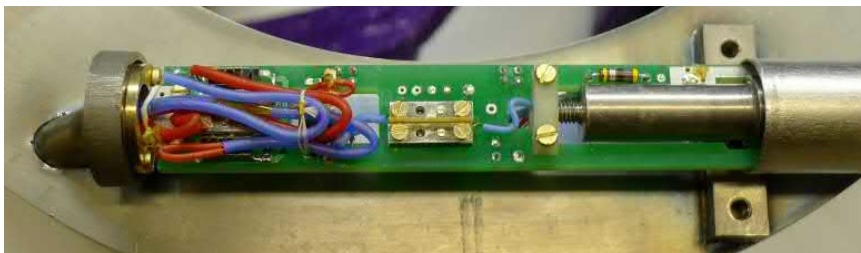
Figure 3.3: SQUID cartridge of a very similar CCC system in operation at CERN. The cartridge encloses the flux transformer and the SQUID sensor, which is protected by an additional shielding can on the right hand side. On the far left the cartridge is connected to the shield enclosing the pick-up coil. Picture taken from [8].
