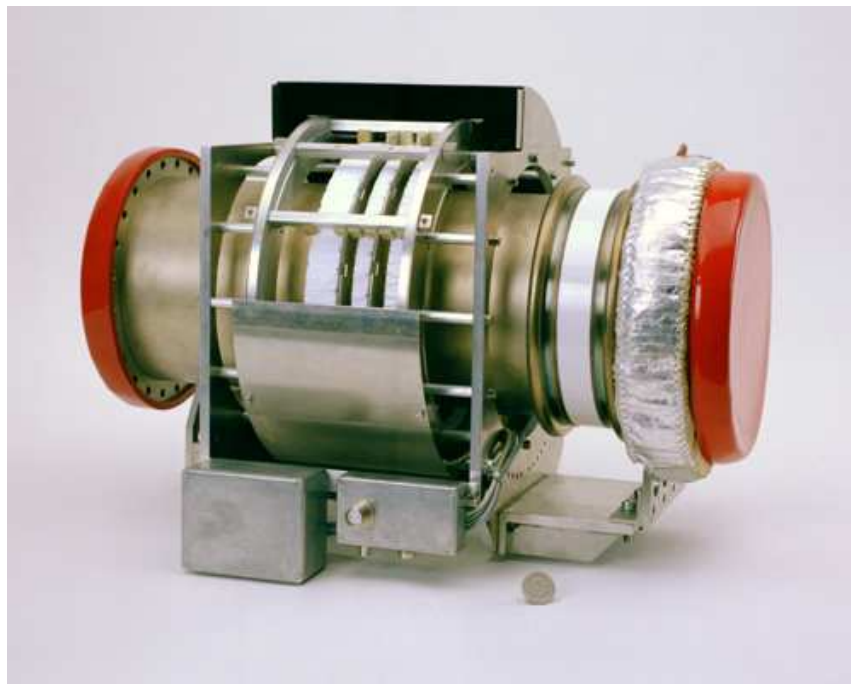
Figure 2.15: The dc-transformer installed at the GSI synchrotron. The left torus is the dc-transformer (two tori mounted closely together), the middle is the ac-transformer used for the feedback of the dc-type and the right one is the ac-transformer for the control of the injection.
