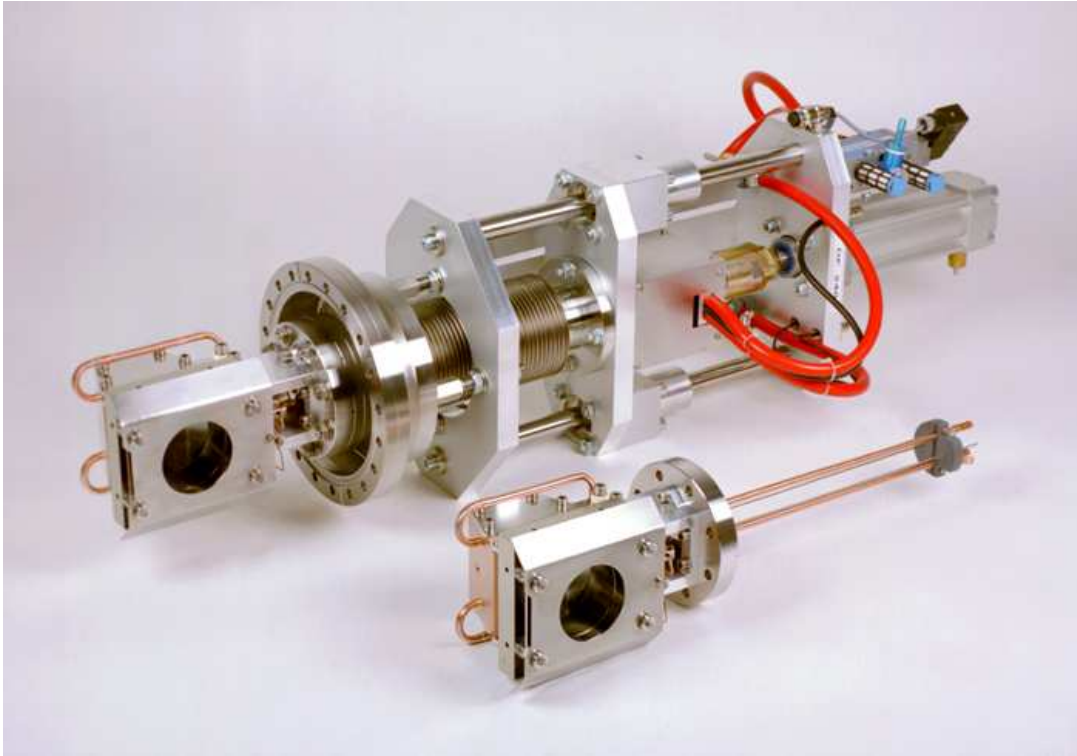
Figure 2.28: Photo of a Faraday cup and beam stopper for high intensity beams as installed at the high current LINAC at GSI. The pneumatic feed-through is mounted on a \varnothing 150 mm flange.
