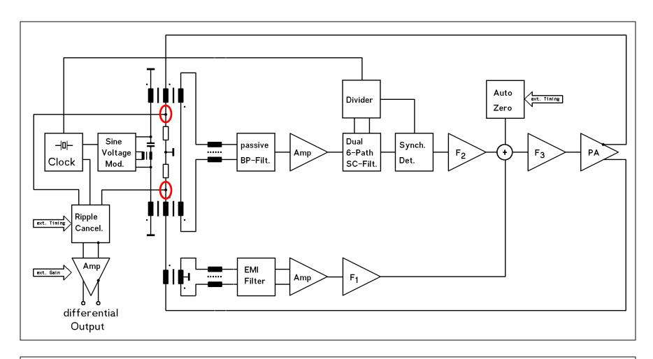
O => differential voltage proportional to DC beam current / U<sub>diff</sub> ~ I<sub>beam</sub>, \* 16.66 V/A, dynamic range ≥ 100 dB
