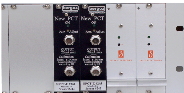
New-PCT Chassis with NPCT-E electronics and power supplies
