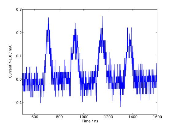
Figure 2: Minimum detectable signal (S/N $\sim$ 3) for the transformer FCT-220-0.50V/A-LLS-H in the HTP beam line. Average charge per pulse  $\sim$ 7.2 pC; total pulse length  $\sim$ 75 ns, peak amplitude 8-10 ADC channels.
