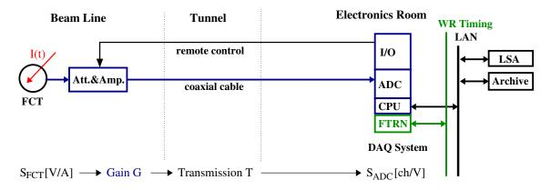
Figure 1: Sketch of data acquisition system. The FCT signal is fed to a front-end hardware consisting of remote-controlled attenuator and amplifier stage. The output is acquired in a sampling ADC after transmission to the electronics room via a coaxial cable.
