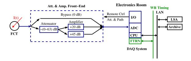
Figure 4: Suggested signal paths for a front-end hardware of a FCT with 0.5 V/A sensitivity. The front-end dynamic range covers [-40,+ 45] dB with a suitable granularity for a  $\pm$  1 Volt ADC input.
