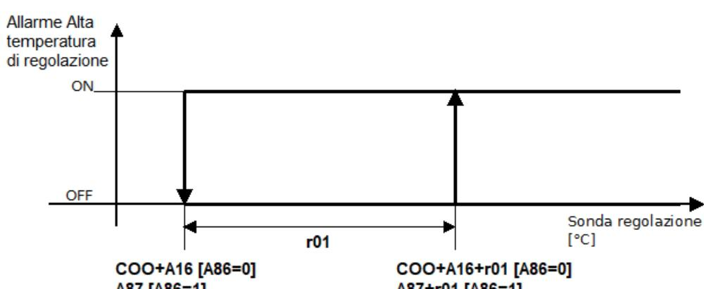
This alarm is generated if the regulation sensor exceeds the value (COO+A16)+r01 if the relative set points are used (A86 = 0), or A87+r01 if the absolute set points are used (A86 = 1) for a time A17. It is cancelled when the regulation sensor falls below the value COO+A16 if the relative set points are used (A86 = 0), or A87 if the absolute set points are used (A86 = 1). Warning only.
