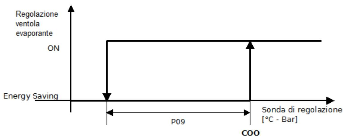
When energy saving mode is set (**P01>0**), when the regulation temperature falls below the value **COO-P09**, the fan alternates 15 seconds of operation with **P01** minutes of inactivity. With each cycle, a check is made that the regulation temperature is below the Set Point (**COO**). Energy saving mode is exited when the regulation temperature reaches the Set Point value (**COO**).
