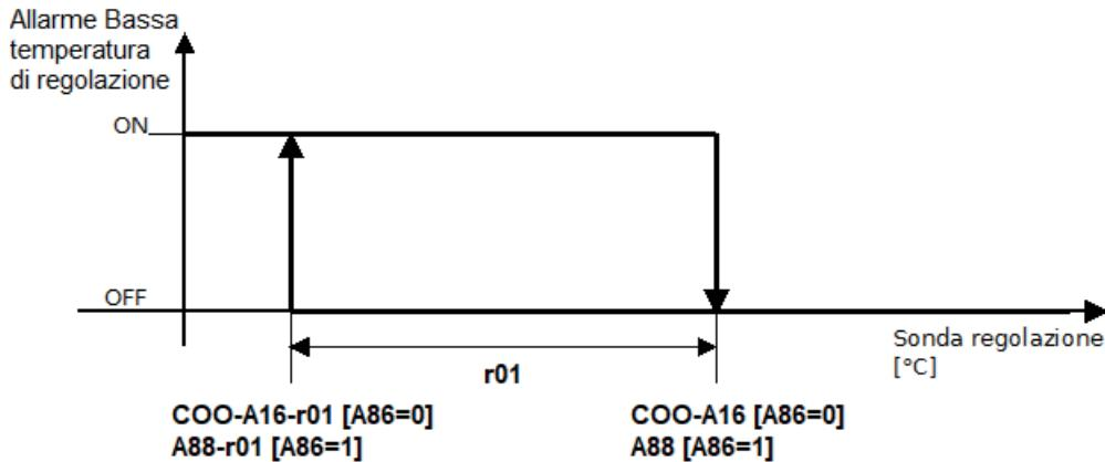
This alarm is generated if the regulation sensor falls below the value (COO-A16)- $r01$  if the relative set points are used (A86 = 0), or A88- $r01$  if the absolute set points are used (A86 = 1) for a time A17. It is cancelled when the regulation sensor reaches the value COO-A16 if the relative set points are used (A86 = 0), or A88 if the absolute set points are used (A86 = 1). Warning only.
