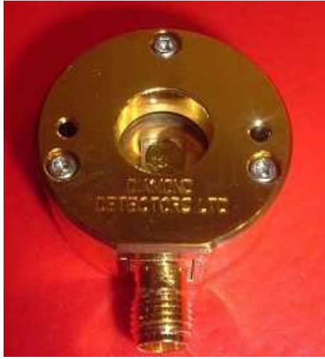
Fig. 3.12: Mono-crystalline diamond detector used for the direct calorimetric measurement and the specification as provided by the manufacturer Diamond Detectors LTD .
