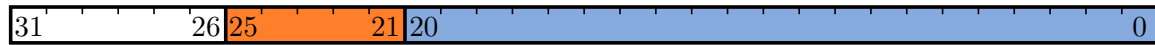
Fig. 4.3: TDC timing represented as a 4-Byte vector. The lower 21-bits contain the actual dump from the internal global clock of the TDC. Given the LSB equivalent of about 24.4 ps, overflowing occurs every 51.2 \mu s
