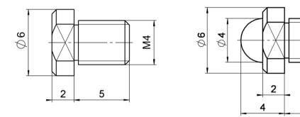
Figure 10: Flat tip (left) and spherical tip (right), dimensions in mm
