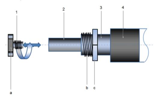
Figure 4: Changing the tip, schematic
