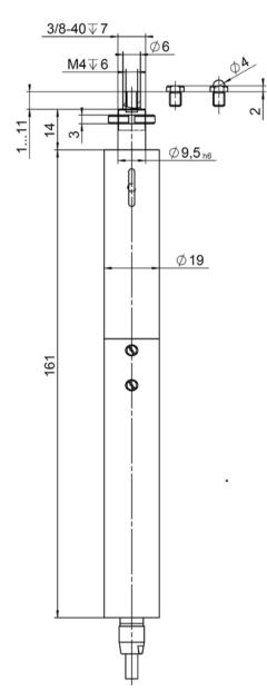
Figure 8: M-230.10, M-230.10S and M-230.10V, dimensions in mm
