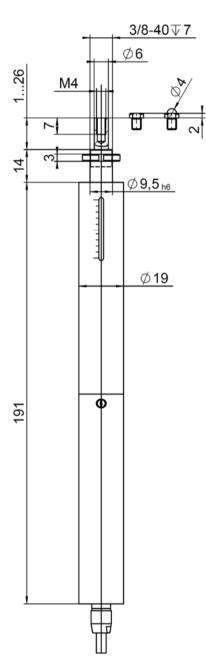
Figure 9: M-230.25, M-230.25S and M-230.25V, dimensions in mm
