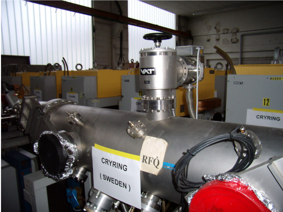
Figure 16: RFQ with connections to out-coupling loops for RF control and reference tank signal for diagnostics. Beam direction right to left.
