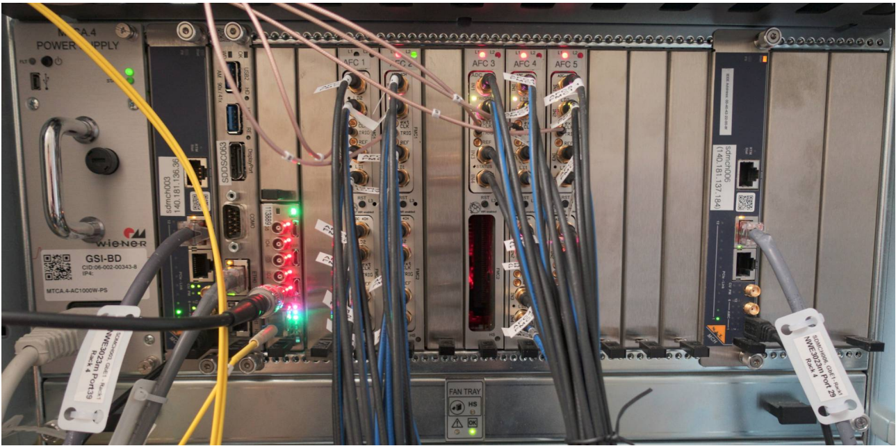
Figure 1.6: MicroTCA crate with from left to right: power supply, MCH, FEC, timing receiver, 5 AFC boards with 9 mounted FMC ADC boards, second MCH
