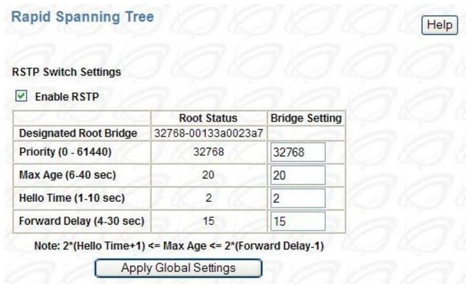
Figure 16: Rapid Spanning Tree
