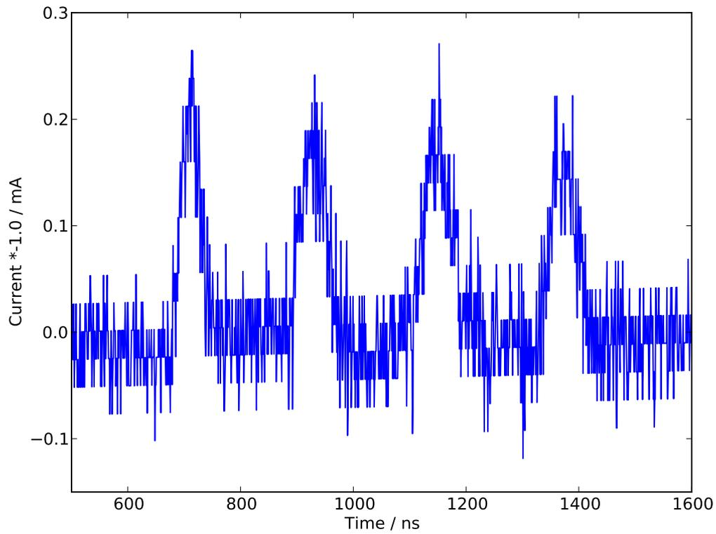
Figure 2: Minimum detectable signal ( $S/N \sim 3$ ) for the transformer FCT-220-0.50V/A-LLS-H in the HTP beam line. Average charge per pulse  $\sim 7.2$  pC; total pulse length  $\sim 75$  ns, peak amplitude 8-10 ADC channels.
