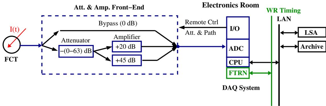
Figure 4: Suggested signal paths for a front-end hardware of a FCT with 0.5 V/A sensitivity. The front-end dynamic range covers  $[-40, +45]$  dB with a suitable granularity for a  $\pm 1$  Volt ADC input.
