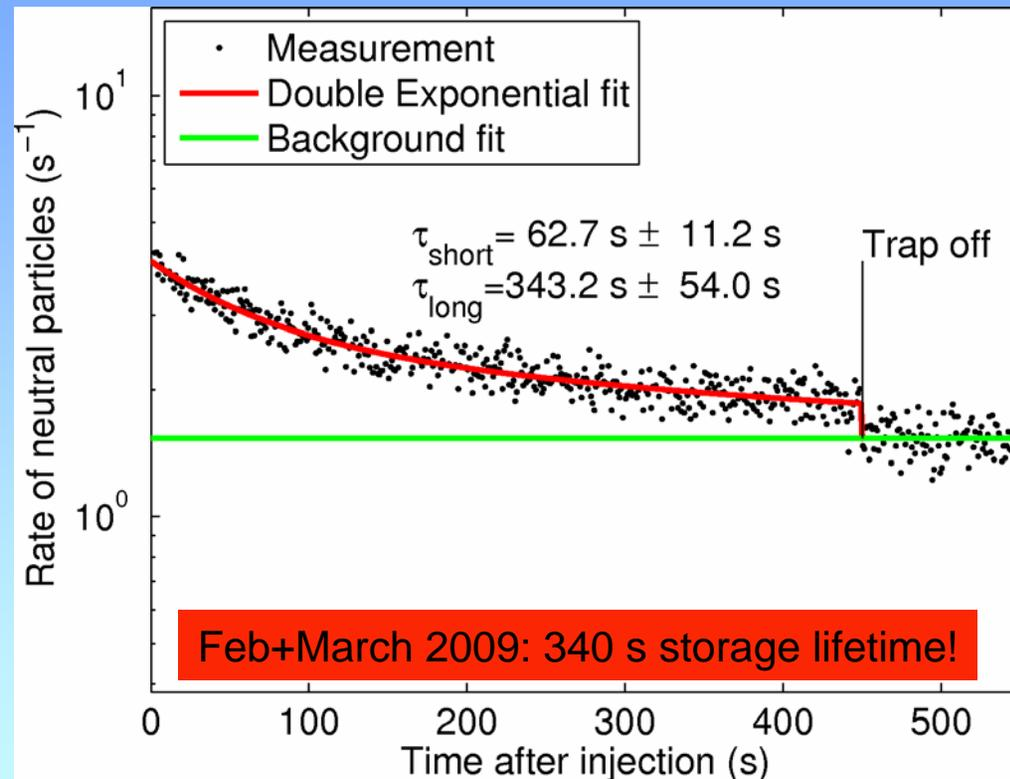
With collision cross-sections from the literature, the new lifetime would translate to a residual gas density of  $44000 \text{ cm}^{-3}$  or  $1.6 \cdot 10^{-12} \text{ mbar}$  (at Room Temperature).
