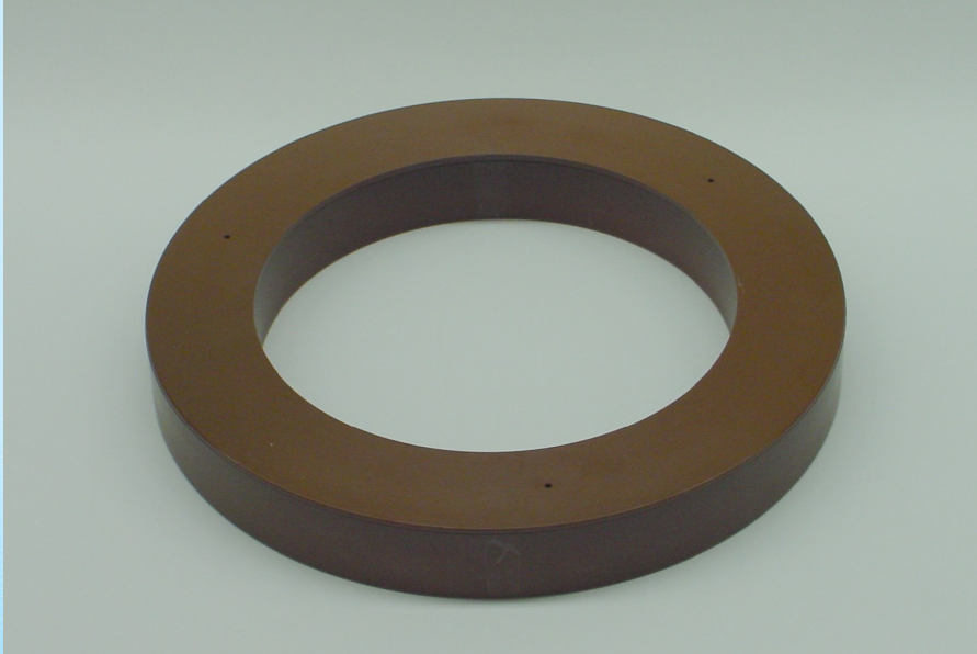
Toroidal core (VITROVAC 6025-F) housed in a VESPEL insulator.
