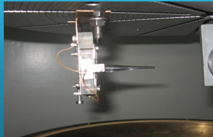
Conical glass capillary and its mounting fixture used in beam focusing experiments
