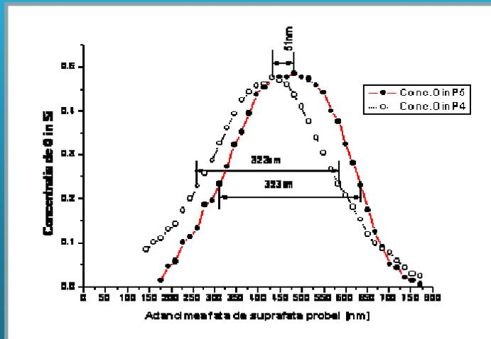
Experimental and simulated RBS spectra and corresponding calculated concentration for a buried oxygen layer in Si before and after thermal annealing at 1000°C
