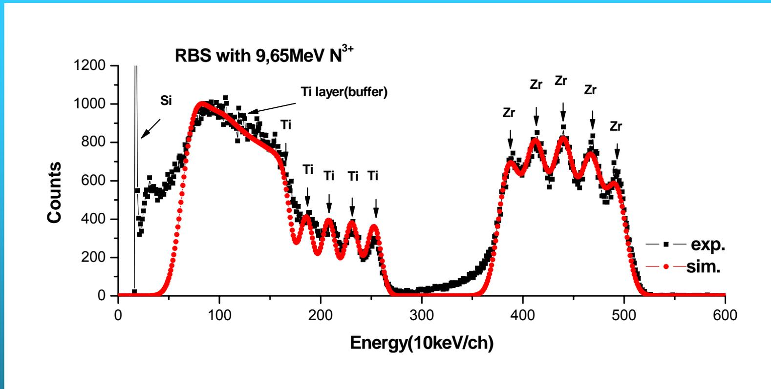
Experimental and simulated spectra for RBS analysis for 5 pairs of ZrN/TiN layers having 15nm/layer deposited on Si with a Ti buffer layer of 300nm obtained using 2.7MeV He beam (before) and 9.65MeV N beam; the use of N beam lead to better mass separation as well as better depth resolution.
