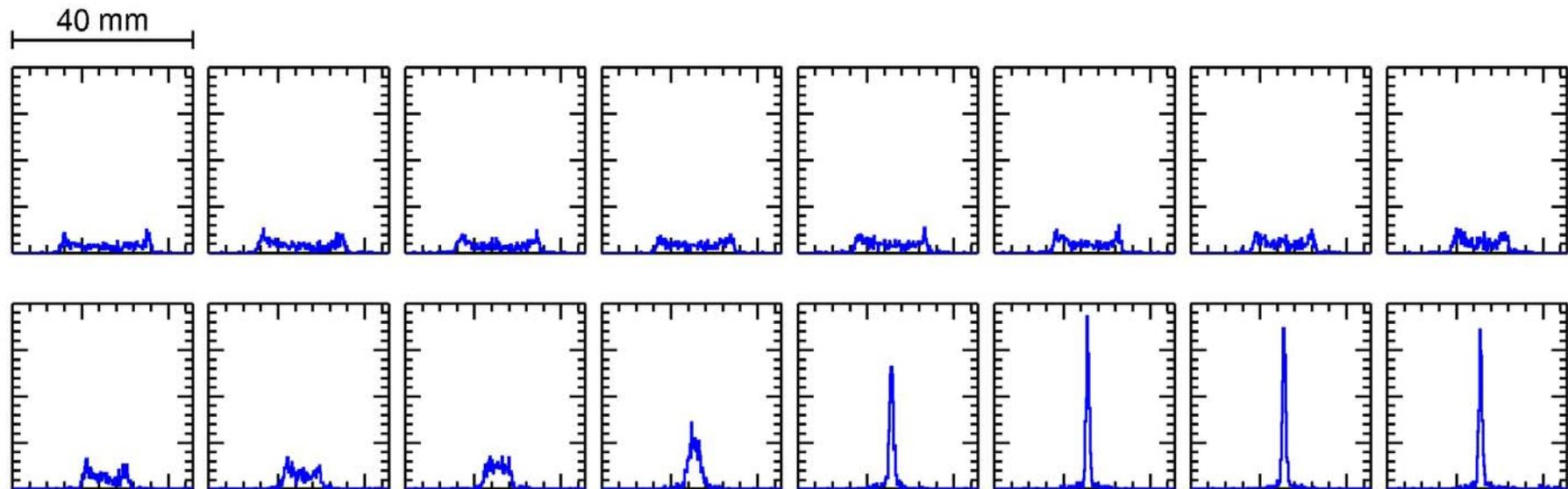
Vertical profiles of an  $F^{6+}$  beam during successive 61-ms intervals, starting 61 ms before the electron beam is realigned with the ion beam and cooling begins.
