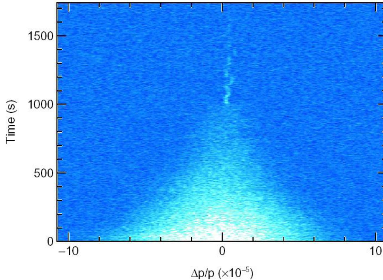
Schottky signal from a beam of  $\text{Xe}^{36+}$  ions showing the transition of the beam to an ordered state at around 1000 particles
