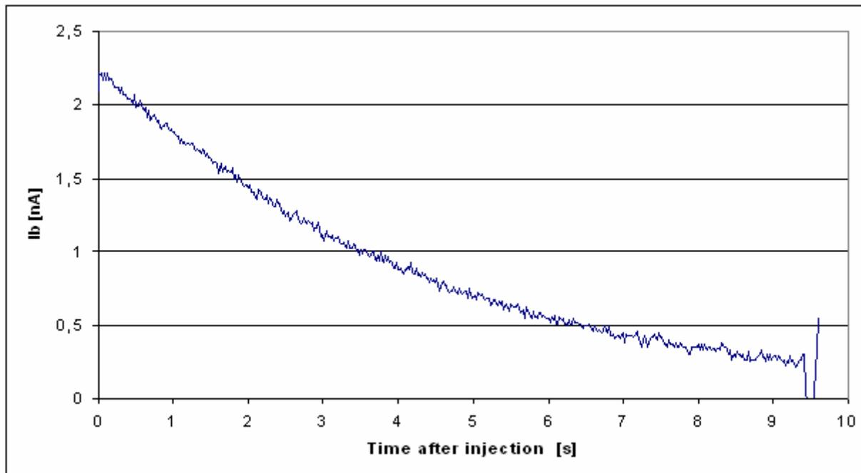
$\text{H}^2\text{S}^+$  bunched beam current during 10 s, averaged over 66 cycles (BW=20 Hz)
