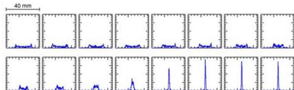
Figure 5: Vertical profiles of an  $\text{F}^{6+}$  beam during successive 61-ms intervals, starting 61 ms before the electron beam is realigned with the ion beam and cooling begins.
