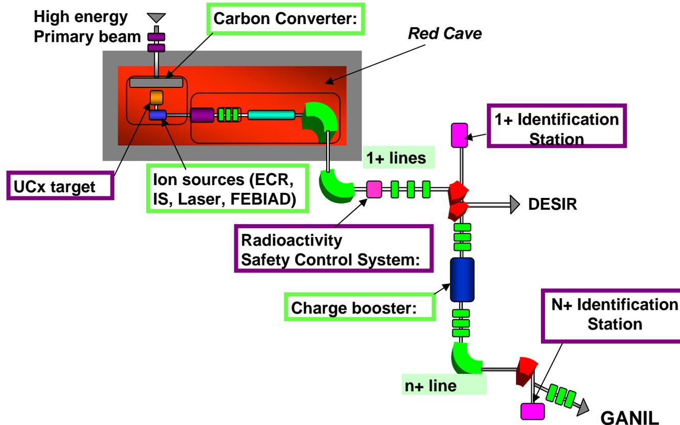
The production of high intensity RIB is based on the fission of an uranium target induced by neutrons. Mono-charged secondary beams are selected in the 1+ beam line, multi ionized to be post accelerated in the existing Ganil.
