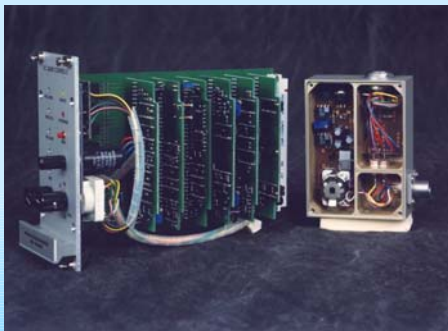
1 channel of the dc SQUID system 5 (left) and the unclosed low noise preamplifier (right).
