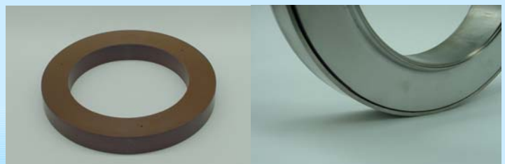
Toroidal core (VITROVAC 6025-F) housed in a VESPEL insulator.
