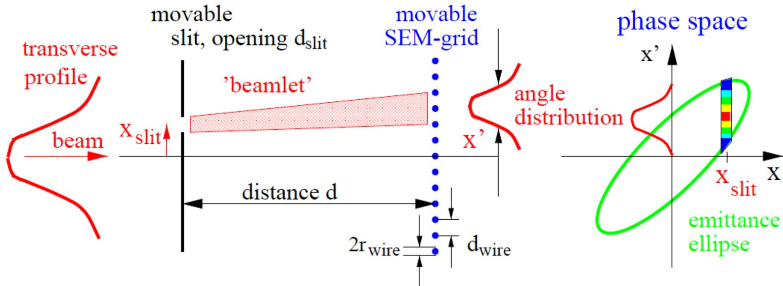
**Slit:** position  $P(x)$  with typical width: 0.1 to 0.5 mm
