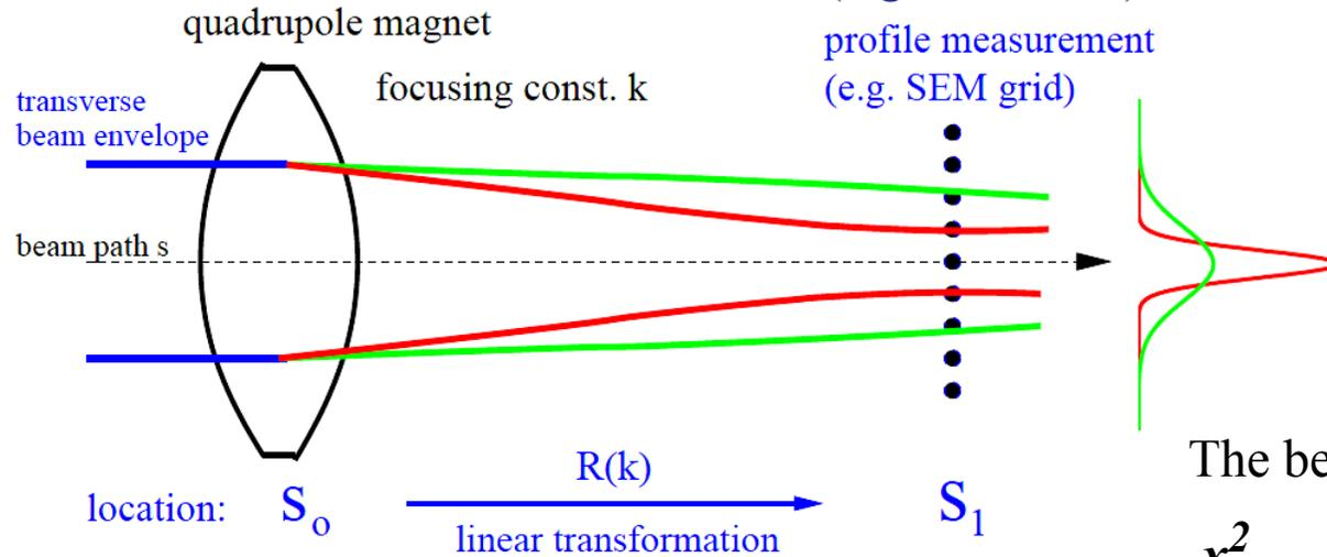
The beam width  $x_{max}$  and  $x_{max}^2 = \sigma_{11}(l, k)$  is measured, matrix  $\mathbf{R}(k)$  describes the focusing.
